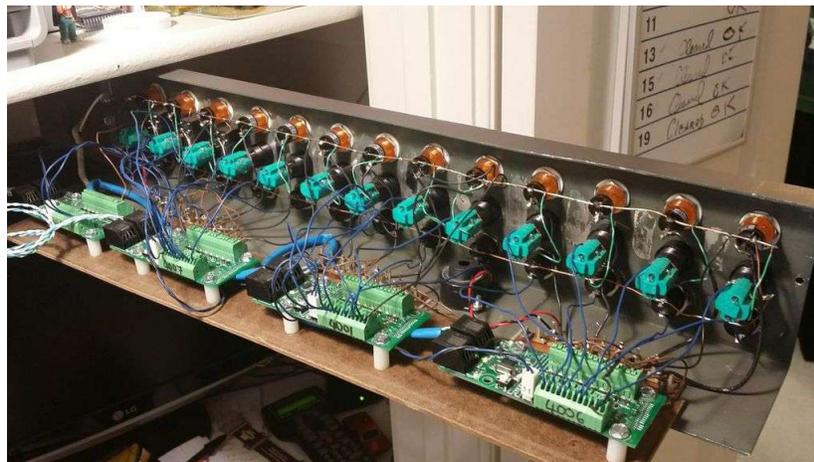
Every "CANBuzz" board can Call and Cancel 4 locations, and all the buzzer lines are connected together to the single buzzer for the Dispatcher.
